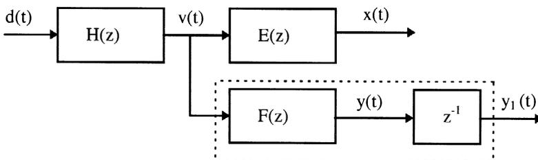
Figure 3. Block diagram to determine equalizer  $\mathbf{e}_1$
