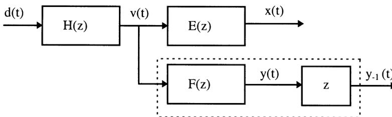
Figure 2. Block diagram to determine equalizer  $\mathbf{e}_{-1}$
