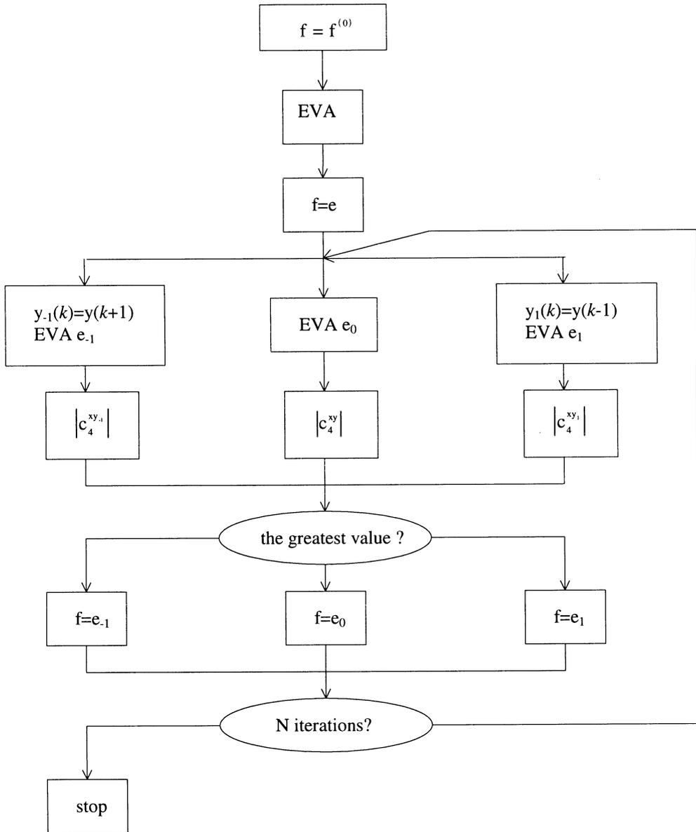
Figure 4. Block diagram of modified iterative EVA procedure
